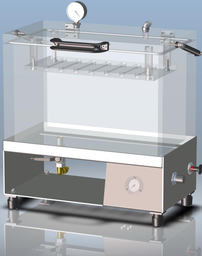
Leak Tester operates on the standard principle of observing the flow of bubbles in water from a leaking pack when under vacuum.
